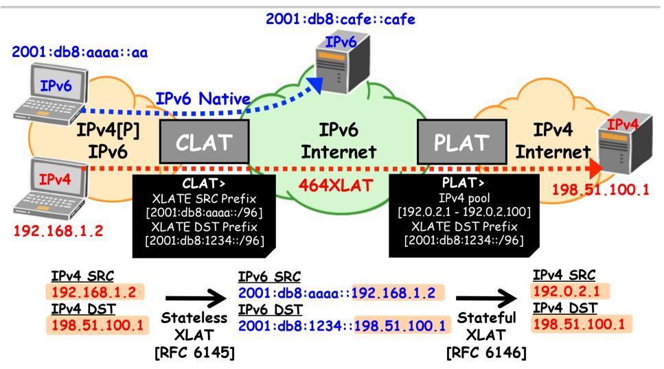
• This architecture consist of CLAT and PLAT have the applicability to wireline network (e.g. xDSL, FTTH) and mobile network (e.g. 3GPP).
