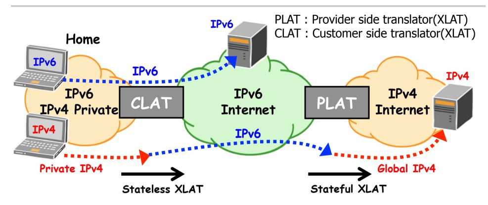
464XLAT provides limited IPv4 connectivity across an IPv6-only network by combining existing and well-known stateful protocol translation RFC 6146 in the core and stateless protocol translation RFC 6145 at the edge.
